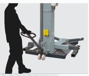
Portable wheels and floating design of rollers make it easy to move the lift. The floating rollers design make the base plate completely contact with ground when lifting with load.
