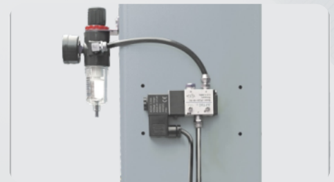
Oil-water separator and Solenoid air valve are installed on the power side column
